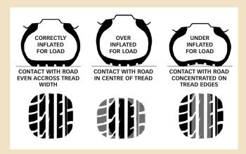
Prolonged under-inflation causes excessive flexing, deterioration of the casing and rapid wear of the tread shoulders. The vehicle will also consume more fuel.
