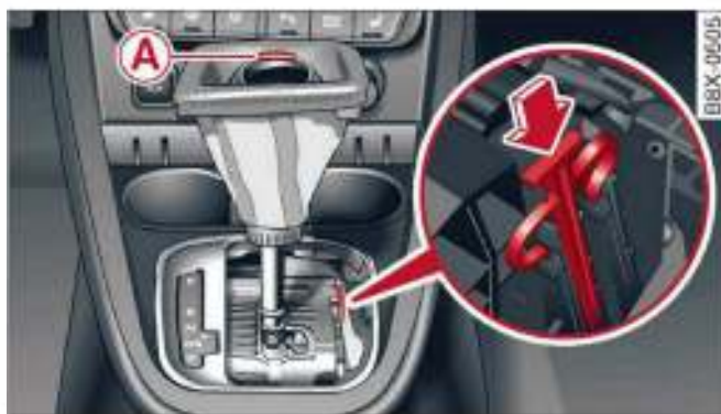
Fig. 84 Manually releasing the selector lever from position P
