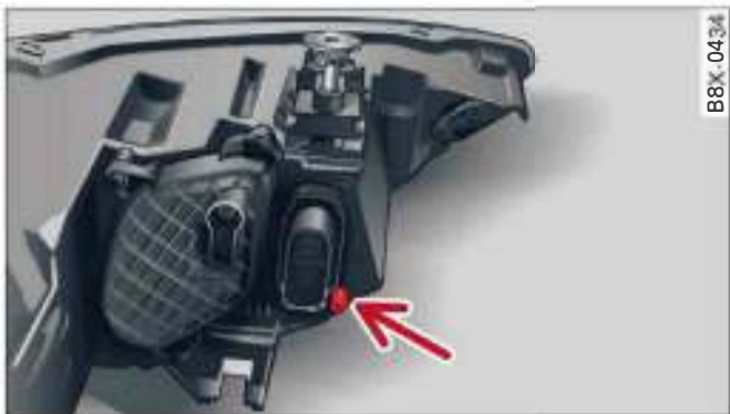
Fig. 199 Headlight unit: Mounting for vent hose
