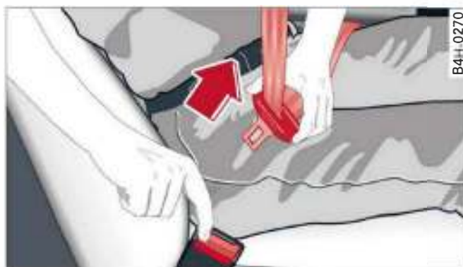
Fig. 120 The latch plate of the belt springs out of the buckle
