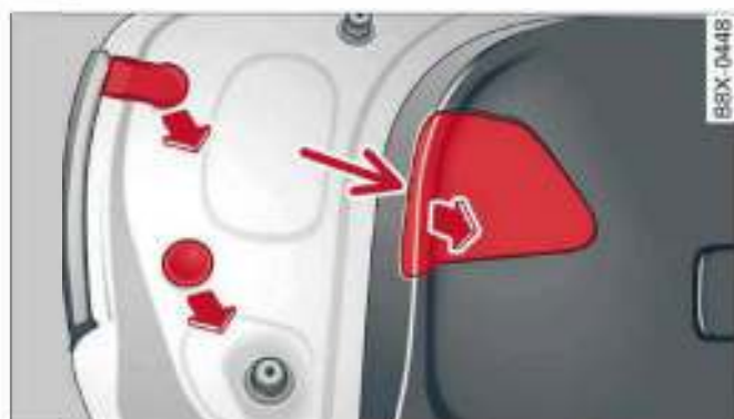
Fig. 204 Boot lid: Location of the retaining screw for the rear light
