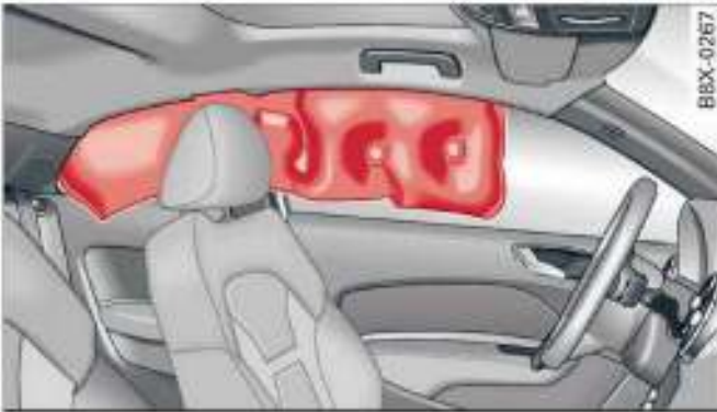
Fig. 130 Head-protection airbags in inflated condition
