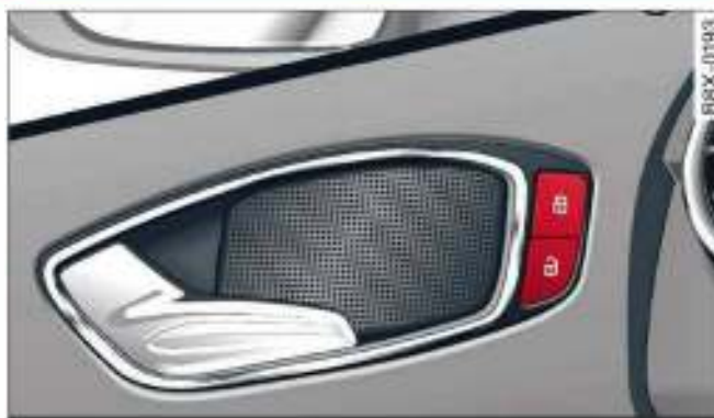
Fig. 25 Driver's door: Central locking switch
