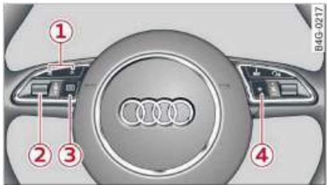
Fig. 11 Multi-function steering wheel: Operating the driver information system
