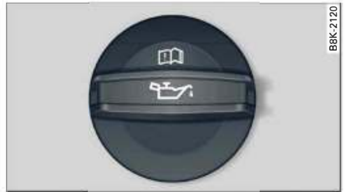
Fig. 140 Engine compartment: Engine oil filler cap
