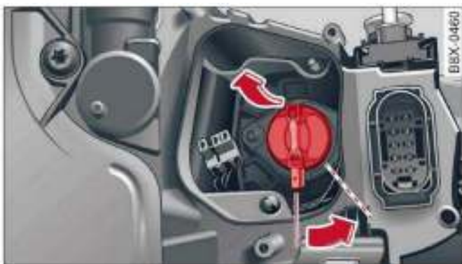
Fig. 190 Bulb housing: Removing the bulb
