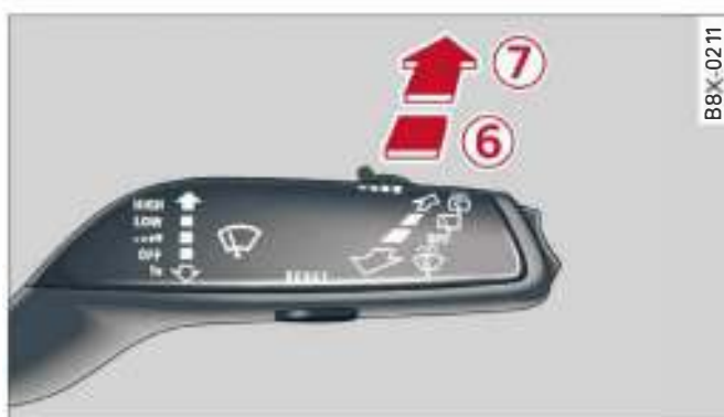
Fig. 44 Windscreen wiper lever: Operating the rear wiper
