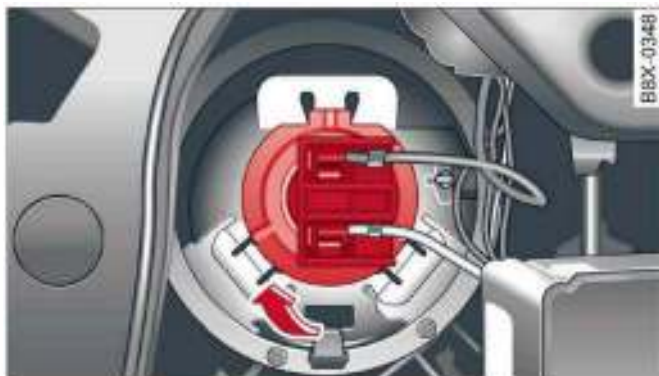
Fig. 186 Bulb housing: Removing bulb for dipped beam headlight
