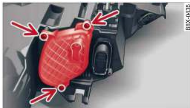
Fig. 188 Headlight: Cover for daytime running lights/side lights/main beam headlights
