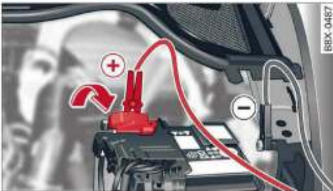
Fig. 143 Version 1) Engine compartment with battery: Terminals for jump leads and battery charger
