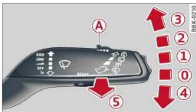
Fig. 43 Windscreen wiper lever: Operating the windscreen wipers
