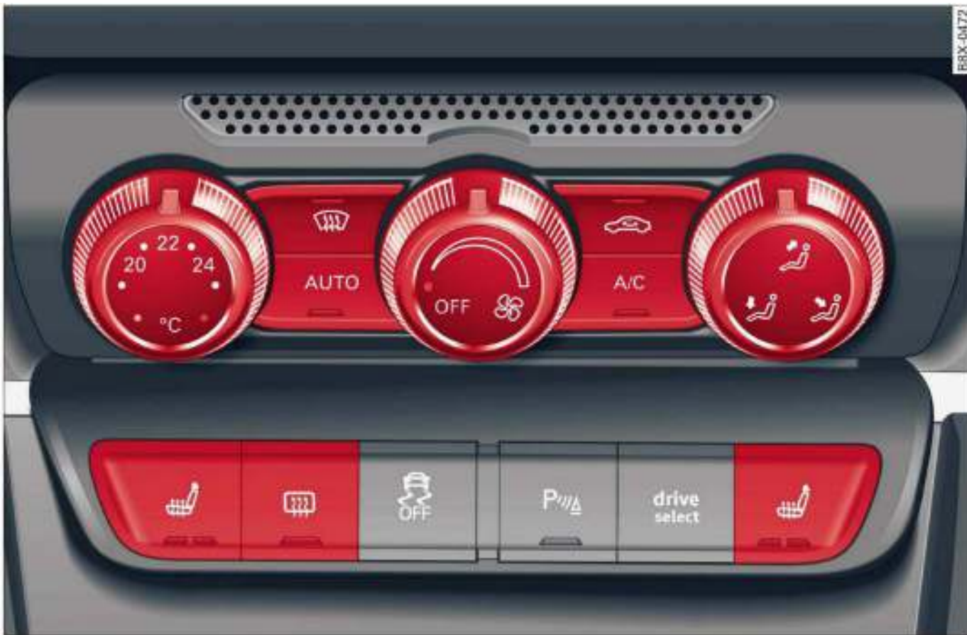
Fig. 70 Centre console: Automatic air conditioner controls
