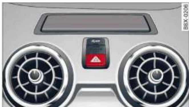
Fig. 36 Dashboard: Switch for hazard warning lights
