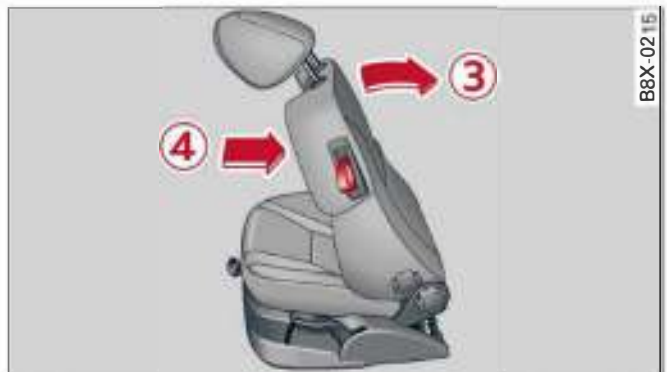
Fig. 49 Driver's seat: Tipping backrest back
