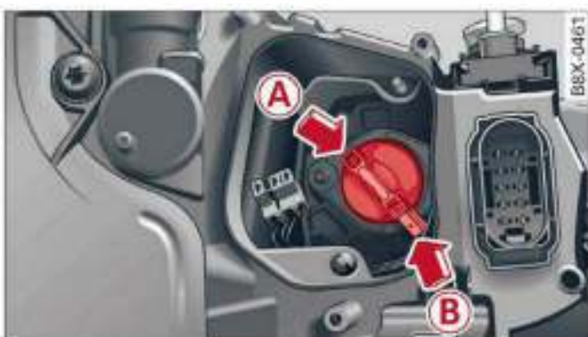
Fig. 191 Bulb housing: Fitting the bulb
