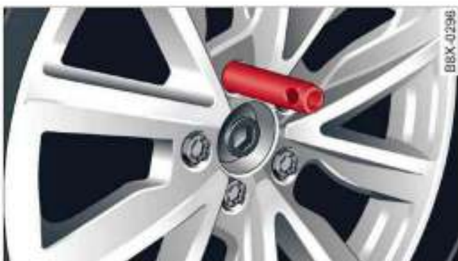
Fig. 164 Wheel: Mounting pin in wheel bolt hole nearest to the top
