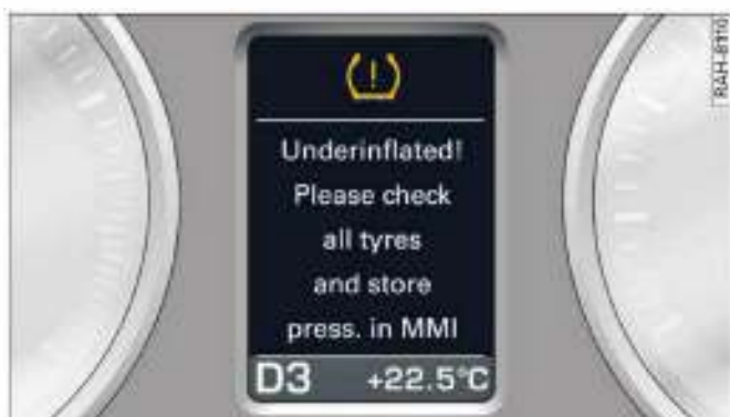
Fig. 148 Instrument cluster: Indicator lamp with message (example)
