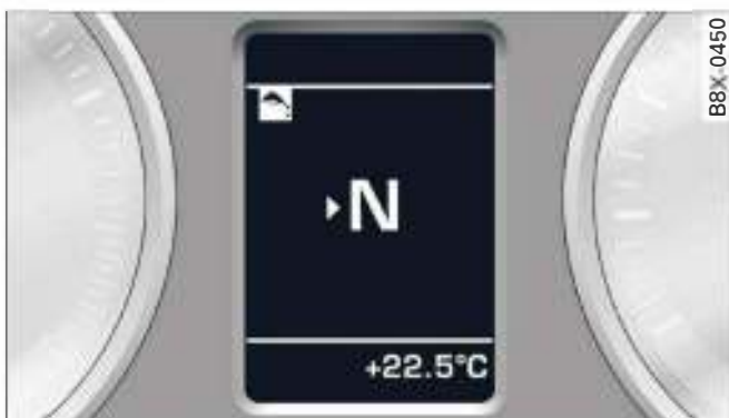
Fig. 15 Instrument cluster: Gear-change indicator recommending neutral
