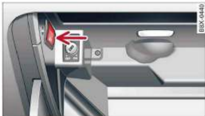
Fig. 149 Glove box: Button for tyre pressure loss indicator
