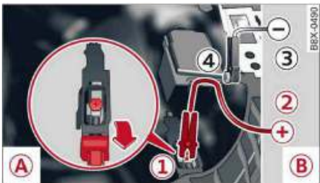
Fig. 171 Version 2) Engine compartment with jump-start terminals: jump-starting with the battery of another vehicle: (A) – Discharged battery, (B) – Boosting battery
