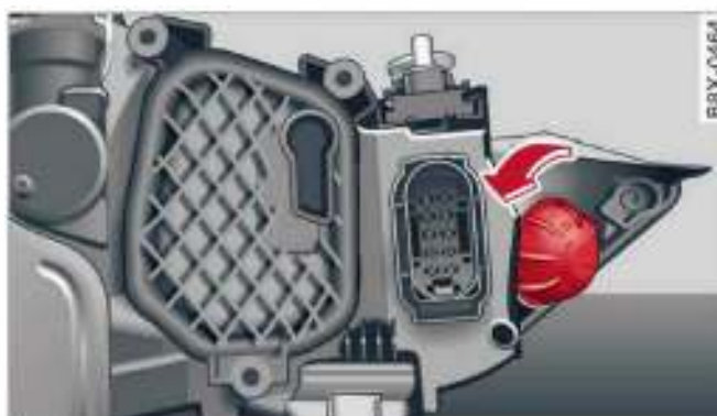
Fig. 193 Headlight: Cover for turn signal
