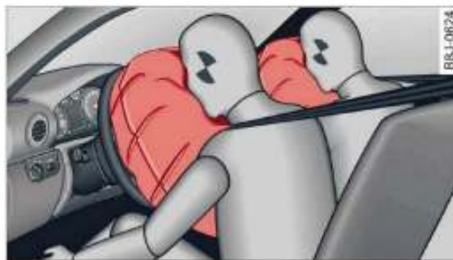
Fig. 125 Front airbags in inflated condition
