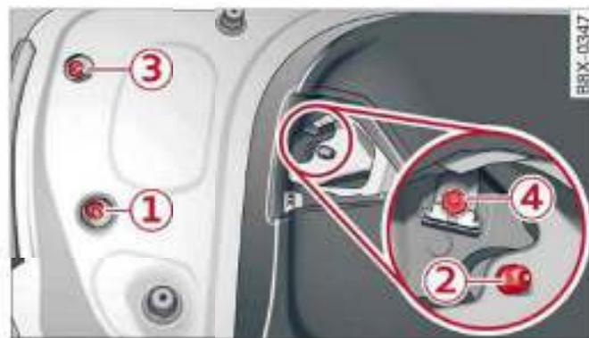
Fig. 210 Boot lid: Location of the retaining screw for the rear light
