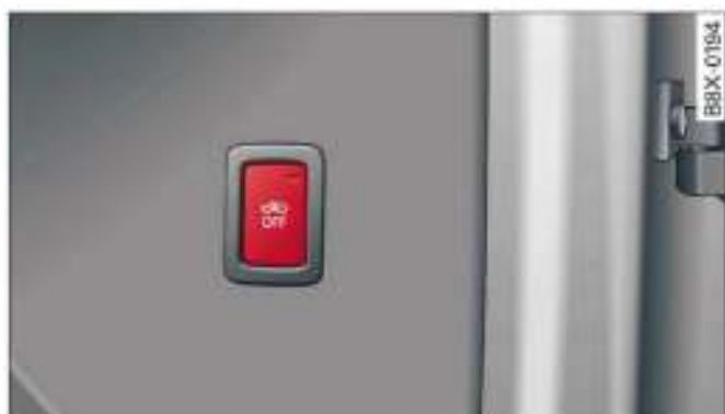
Fig. 27 End face of (open) driver's door: Button for interior monitor/tow-away protection
