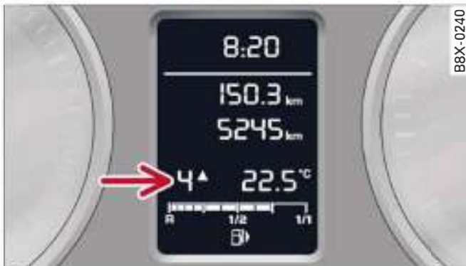
Fig. 6 Instrument cluster: Gear-change indicator on vehicles without driver information system
