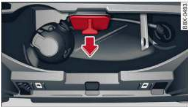
Fig. 89 Area below rear bumper: Pulling out plug
