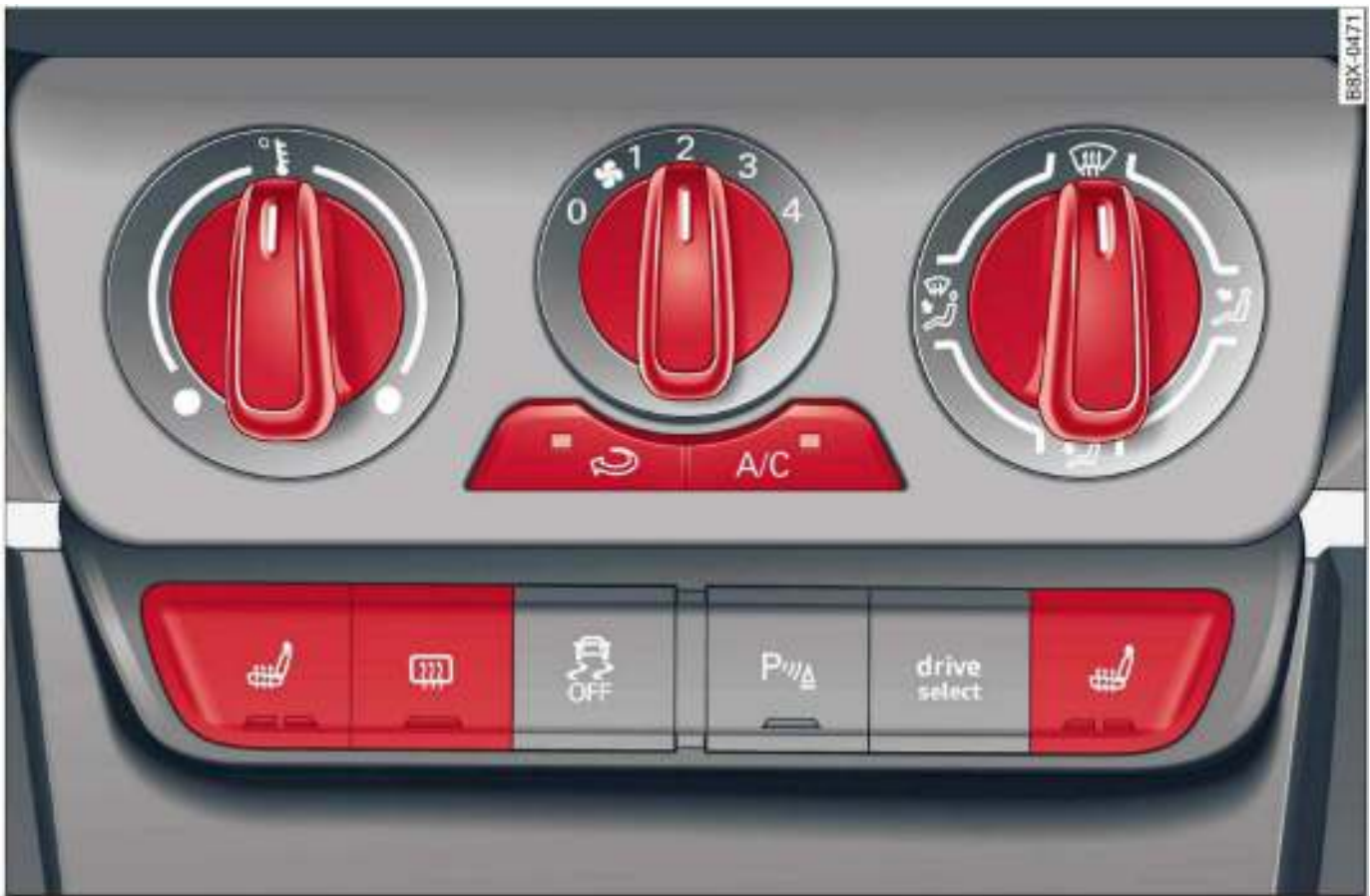
Fig. 69 Centre console: Controls for the heating/ventilation system and manual air conditioner
