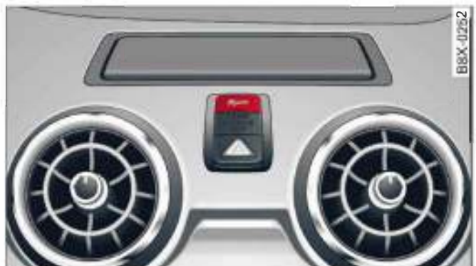
Fig. 76 Dashboard: Switch for start/stop system
