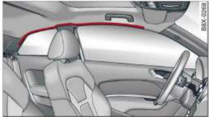
Fig. 129 Location of head-protection airbags above the doors
