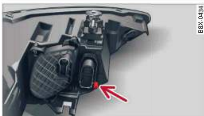
Fig. 184 Headlight unit: Mounting for vent hose
