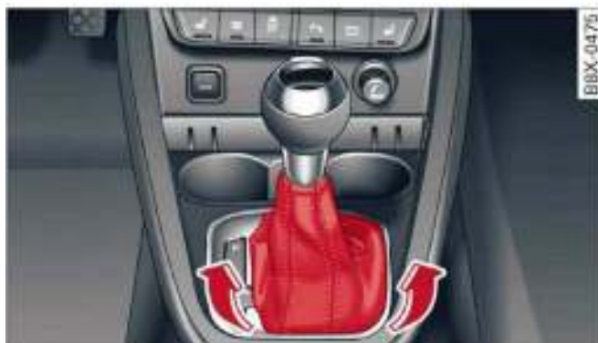
Fig. 83 Selector lever: Removing the cover
