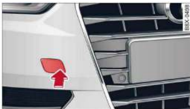
Fig. 172 Right side of the front bumper: Removing the cap
