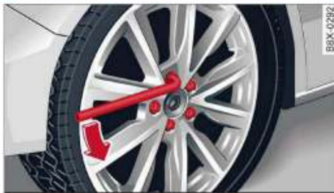
Fig. 160 Wheel: Loosening the wheel bolts
