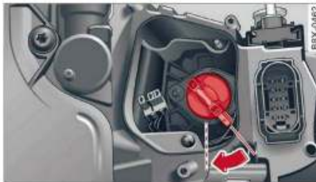
Fig. 192 Bulb housing: Fitting the bulb
