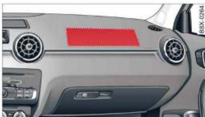
Fig. 124 Front passenger's airbag in dashboard
