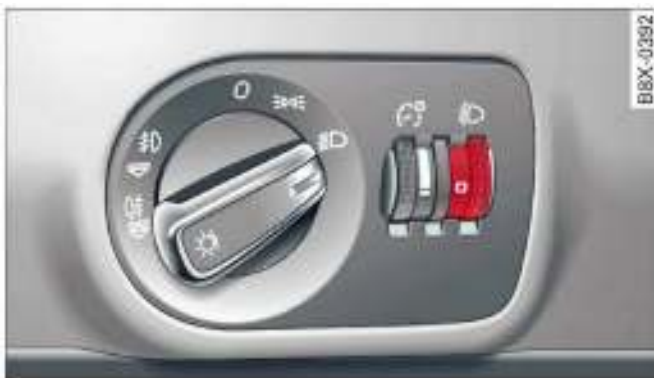
Fig. 34 Dashboard: Light switch with headlight range control
