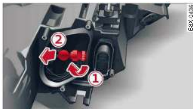
Fig. 197 Bulb housing: Removing bulb for turn signal
