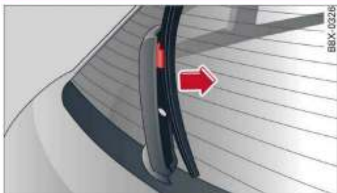
Fig. 46 Rear window wiper: Taking off the wiper blade
