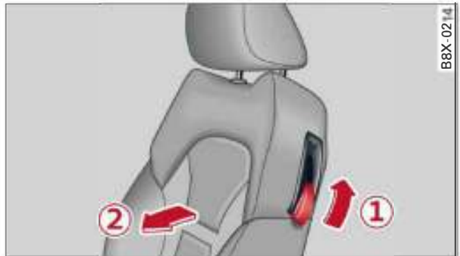
Fig. 48 Driver's seat: Unlocking backrest
