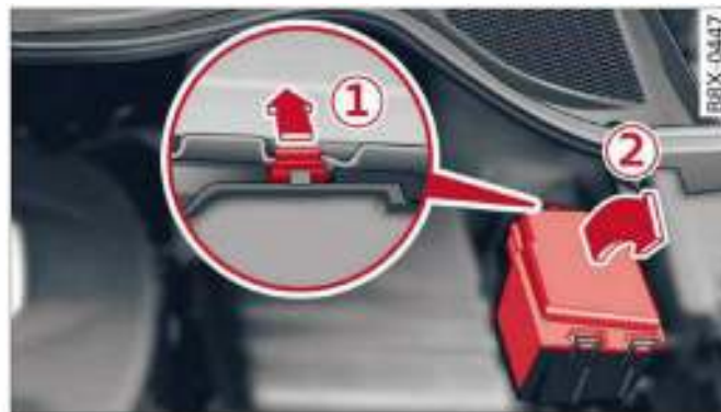
Fig. 179 Engine compartment: Releasing cover
