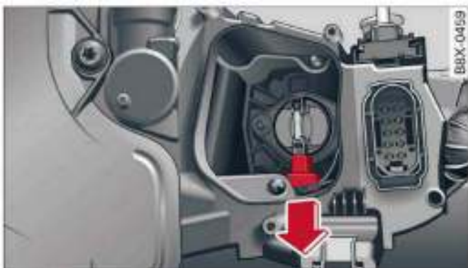
Fig. 189 Bulb holder: Removing the plastic connector
