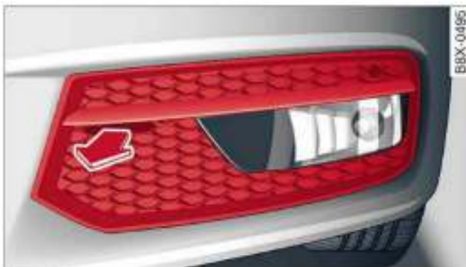
Fig. 200 Front fog light: Removing trim
