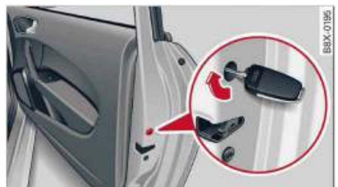
Fig. 26 Passenger's door/rear door: Locking manually
