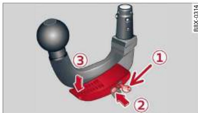
Fig. 93 Removable towing bracket: Removing the ball joint
