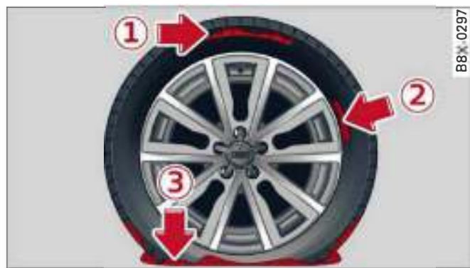
Fig. 155 Tyres: Irreparable tyre damage
