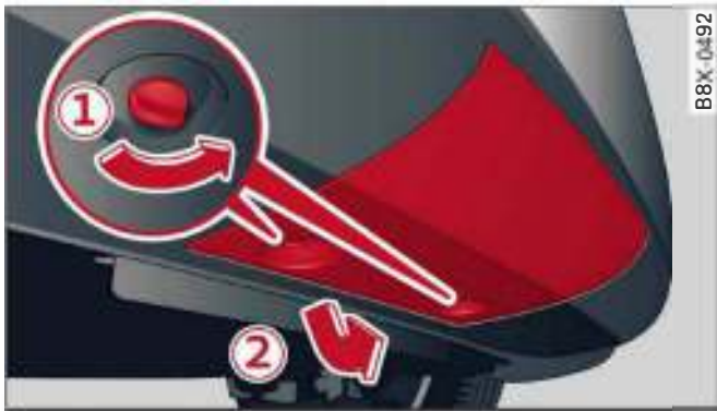
Fig. 88 Area below rear bumper: Removing bumper cover
