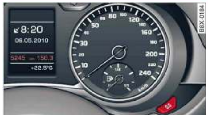
Fig. 4 Instrument cluster: Mileage recorder and reset button
