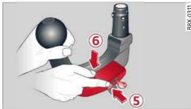
Fig. 87 Removable towing bracket: Setting the spring mechanism to the "ready" position
