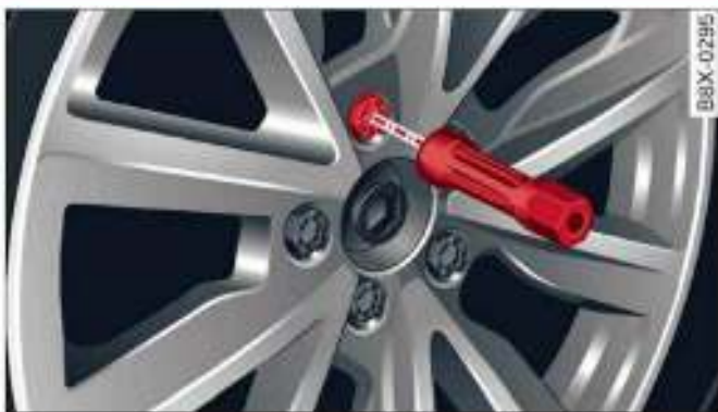
Fig. 163 Wheel: Hexagonal socket for turning wheel bolts
