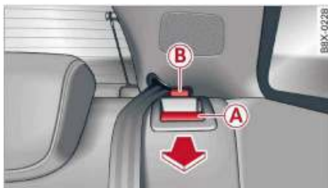
Fig. 61 Backrest: Release lever (example of left side)
