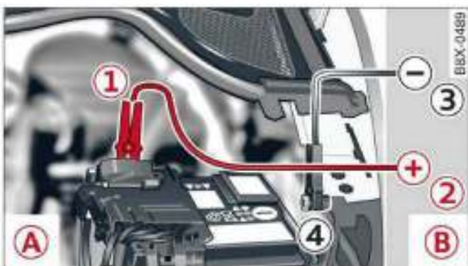
Fig. 170 Version 1) Engine compartment with battery: jump-starting with the battery of another vehicle: (A) – Discharged battery, (B) – Boosting battery
