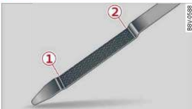
Fig. 139 Oil dipstick (example): Checking engine oil level
