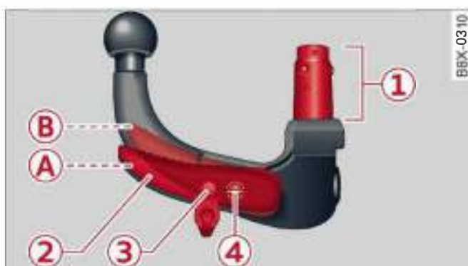
Fig. 86 Removable towing bracket: Requirements for fitting ball joint
