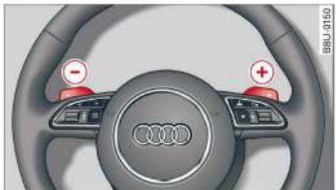
Fig. 82 Steering wheel: Manual gear selection with paddle levers*
