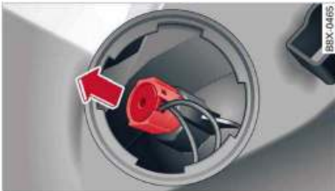
Fig. 194 Bulb housing: Removing bulb for turn signal
