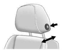
To adjust the head restraint forward or rearward, press the button located on the side facing of the head restraint and move it forward or rearward until the desired locking position is reached. Try to move the head restraint after the button is released to make sure that it is locked in place.
