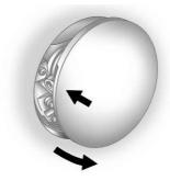
The fuel cap is behind a hinged fuel door on the passenger side of the vehicle. To open the fuel door, push and release the rearward center edge of the door. If equipped, the fuel door is locked when the vehicle doors are locked. Press on the RKE transmitter to unlock.
