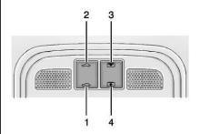
On vehicles with a sunroof, the switch is on the overhead console.
