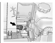
The vehicle has a remote positive (+) terminal under a trim cover. It is under the battery cover on the driver side of the engine compartment. See *Engine*Compartment Overview
