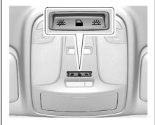
: Turns the lamps on when any door is opened.
