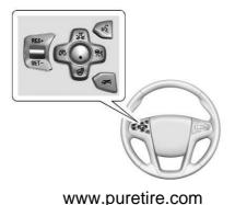
(On/Off): Press to turn the system on or off. The indicator turns white on the instrument cluster when ACC is turned on.
