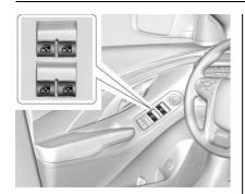
Press the switch to lower the window. Pull the switch up to raise it.
