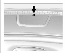
The indicator light, on the instrument panel near the windshield, indicates the status of the system.
