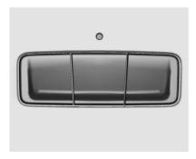
If equipped, these buttons in the overhead console provide a way to replace up to three remote control transmitters used to activate devices such as garage door openers, security systems, and home automation devices.
