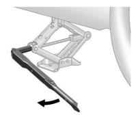
Turn the jack handle clockwise to raise the vehicle far enough off the ground for the compact spare to fit under the vehicle. 294
