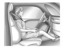
If a person of adult-size is sitting in the front outboard passenger seat, but the off indicator is lit, it could be because that person is not sitting properly in the seat. Use the following steps to allow the system to detect that person and enable the front outboard passenger frontal airbag:
