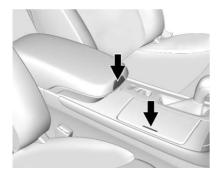
There is storage in the center console armrest. Press the button to access. Depending on the options, there may be an accessory power outlet, auxiliary jack, USB port(s), and a transmitter pocket inside. See *Power Outlets* \$\dip 103\$ and the infotainment manual.
