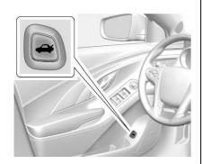
To open the trunk, press on the driver door when the vehicle is off or in P (Park).
