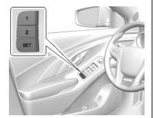
If equipped, the 1, 2, and SET buttons on the driver door are used to manually store and recall the driver seat, and outside mirror positions.
