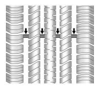
Treadwear indicators are one way to tell when it is time for new tires. Treadwear indicators appear when the tires have only 1.6 mm (1/16 in) or less of tread remaining. See Tire
