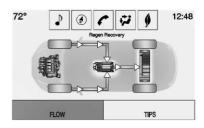
Regen Recovery – Power from the wheels returns to the battery during regenerative braking or coasting.
