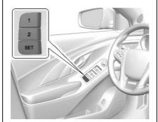
If memory equipped, the 1, 2. and SET buttons on the driver door are used to manually store and recall the driver seat and outside mirror positions.
