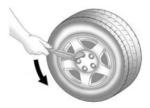
Turn the wheel wrench counterclockwise to loosen all of the wheel nuts, but do not remove them yet.
