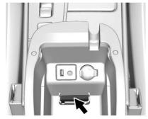
Place the new transmitter into the transmitter pocket inside the armrest storage area.
