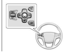
(On/Off): Press to turn cruise control on or off. A white indicator comes on in the instrument cluster.
