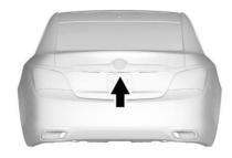
To open the trunk from outside the vehicle, press and hold HOLD on the Remote Keyless Entry (RKE) transmitter to unlock all doors, then use the touchpad above the license plate. If equipped with Keyless Access, the trunk can be opened using the touchpad when the RKE transmitter is within 1 m (3 ft) of the rear of the vehicle.
