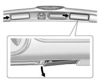
Push the end on either of the lamp assemblies (passenger side shown) and then move the lamp assembly down to remove it from the trunk lid.
