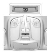
If equipped, the rear window sunshade button is on the overhead console. To open the sunshade, press and release. The sunshade will fully extend. To close the sunshade, press and release the switch again. The sunshade will fully close.
