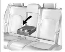
The rear seat has an armrest in the center of the seatback. Lower the armrest to access the two cupholders and the storage area.
