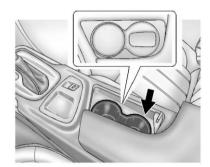
Place the new transmitter into the transmitter pocket with the buttons facing up. The transmitter pocket is located inside the center console
