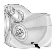
Vehicles with an automatic transmission are equipped with an electronic key lock release system. This system is to prevent ignition key removal unless the shift lever is in P (Park).
