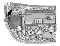
The electrical cord is located on the passenger side of the engine compartment, between the fender and the air cleaner. 3. Plug it into a normal, grounded 110-volt AC outlet.
