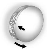
The tethered fuel cap is behind the fuel door on the vehicle's passenger side. Turn the fuel cap counterclockwise to remove. Reinstall the cap by turning it clockwise until it clicks.
