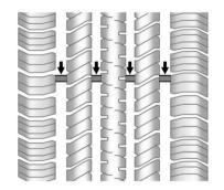
Treadwear indicators are one way to tell when it is time for new tires. Treadwear indicators appear when the tires have only 1.6 mm (1/16 in) or less of tread remaining. See *Tire Inspection on page 10-54* and *Tire Rotation on page 10-55*.
