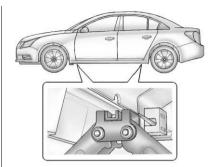
Position the jack lift head at the jack location nearest the flat tire. The location is indicated by a mark near the bottom edge of the lower molding. The jack must not be used in any other position.
