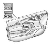
The power window switches are located on the driver door. Each passenger door has a switch that controls only that window.
