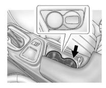
Place the transmitter in the transmitter pocket with the buttons facing up. 3. With the vehicle in P (Park) or N (Neutral), press the brake pedal and the START STOP button. See Starting the Engine on page 9-19 for additional information about the vehicle's keyless ignition with pushbutton start.
