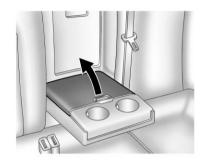
Pull down the armrest. Push the button to lift the cover. Close the cover before folding the armrest up.
