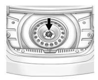
Turn the retainer nut counterclockwise and remove the spare tire. Place the spare tire next to the tire being changed.  The jack and tools are stored below the spare tire. Remove them from their container and place them near the tire being changed.
