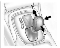
DSC allows you to shift an automatic transmission similar to a manual transmission. To use the DSC feature:
