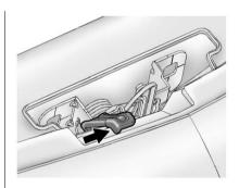
Go to the front of the vehicle and move the secondary hood release handle to the right.
