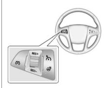
(Heated Steering Wheel): For vehicles with a heated steering wheel, press to turn on or off. A light on the button displays when the feature is turned on.
