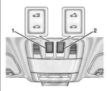
For vehicles with a sunroof, the sunroof only operates when the ignition is in ON/RUN or ACC/
