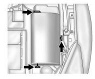
To remove the fuse block cover, press the three retaining clips on the cover and lift it straight up.
