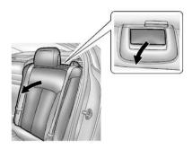
Pull on the lever on the top of the seatback to unlock it.
