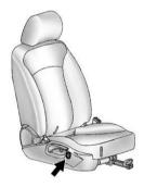
Press and hold the top or bottom of the switch to raise or lower the seat. Release the switch when the desired height is reached.
