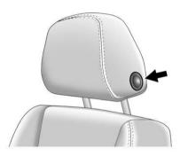
To raise or lower the head restraint, press the release button located on the side of the head restraint and pull up or push the head restraint down and release the button.
