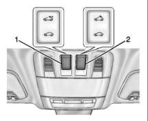
For vehicles with a sunroof, the sunroof only operates when the ignition is in ON/RUN or ACC/ ACCESSORY or in Retained Accessory Power (RAP). See Retained Accessory Power (RAP) on page 9-23.
