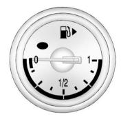
When the ignition is on, the fuel gauge shows about how much fuel is left in the tank.
