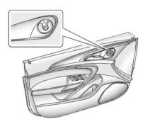
Controls for the outside power mirrors are located on the driver door.
