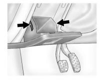
The instrument panel fuse block is located in the instrument panel, on the driver side of the vehicle.
