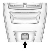
The power outlet is on the rear of the center console.
