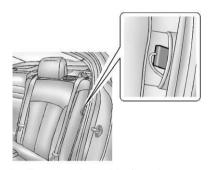
Remove the guide from its storage pocket on the side of the seat.
