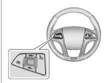
ৈ (On/Off): Press to turn the cruise control system on and off. An indicator light will turn on or off in the instrument cluster.
