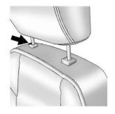
Pull the head restraint up to raise it. To lower the head restraint, press the release button, located on the head restraint post on the top of the seatback, while you push the head restraint down.
