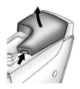
Push the button to access the storage or accessory power outlet under the armrest. See *Power Outlets on page 5-6*.
