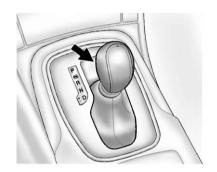
The automatic transmission has a shift lever located on the console between the seats
