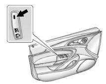
Press at to activate the safety locks on the rear doors. The indicator light will illuminate.
