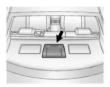
The eAssist system high voltage battery is cooled with air drawn from the vehicle interior. The cold air
