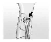
Press down on the release button and move the height adjuster to the desired position. After the adjuster is set to the desired position, try to move it down without pushing the release button to make sure it has locked into position.
