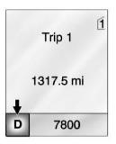
The mode or selected gear is shown in the instrument cluster.
