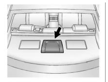
The cold air intake for the battery is located behind the rear seat, on the filler panel. Do not cover the intake. See *Battery on page 10-26*.
