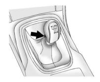
This is the shift pattern for the six-speed manual transmission.
