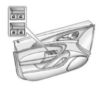
The power window switches located on the driver door control all four windows. The passenger doors have a window switch that controls that window. Push the switch down to open the window. Pull the front of the switch up to close it.
