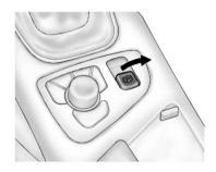
The vehicle has an Electric Parking Brake (EPB). The switch for the EPB is on the center console. The EPB can always be activated, even if the ignition is off. To prevent draining the battery, avoid repeated cycles of the EPB system when the engine is not running.
