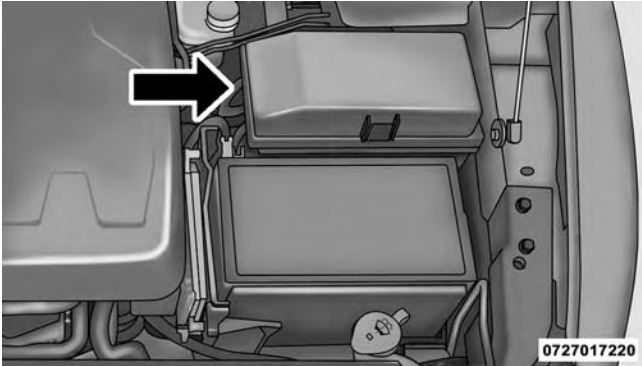
Power Distribution Center
