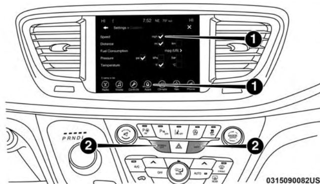
Uconnect 8.4 Buttons On The Touchscreen And Buttons On The Faceplate
