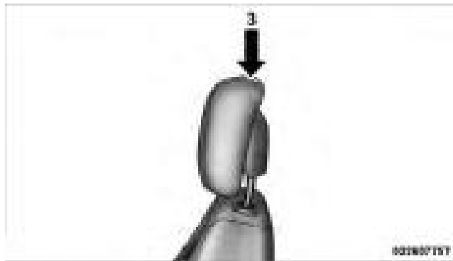
3 — Final Downward Movement To Engage Locking Mechanism
