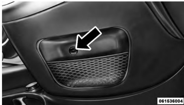
Shift Lever Override Access Hole
