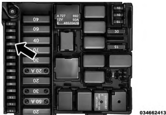
Power Outlet Fuse Location Underhood
