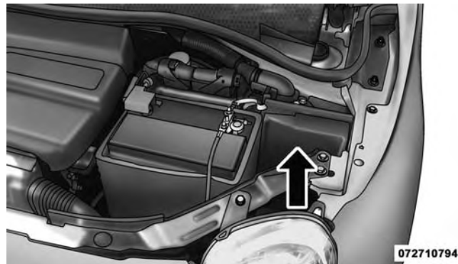
Front Distribution Unit
