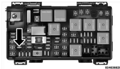
Power Outlet Fuse Location
