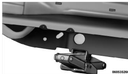
Front Jacking Location
