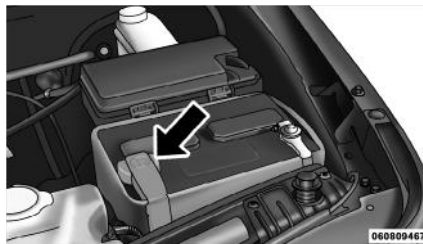
Positive Battery Post
