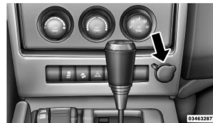
Front Power Outlet
