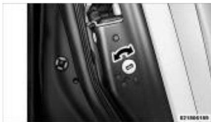
Child-Protection Door Lock Function
