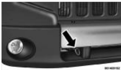
Front Tow Eye Installed
