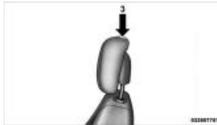
3 — Final Downward Movement To Engage Locking Mechanism
