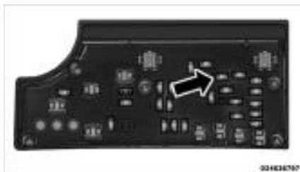
Power Outlet Fuse Location
