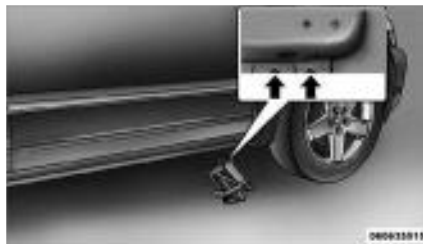
Front Jacking Location
