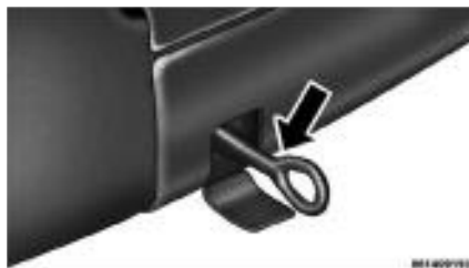
Rear Tow Eye Installed
