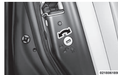
Child-Protection Door Lock Function
