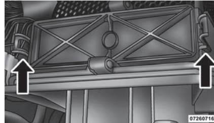
A/C Air Filter Replacement
