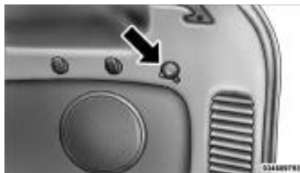
Rear Power Outlet
