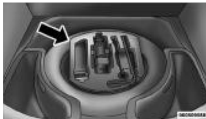
Jack Storage Location
