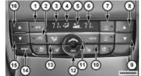
Automatic Temperature Control (ATC) Panel
