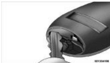
Separating RKE Transmitter
