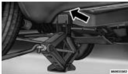
Front Jacking Location
