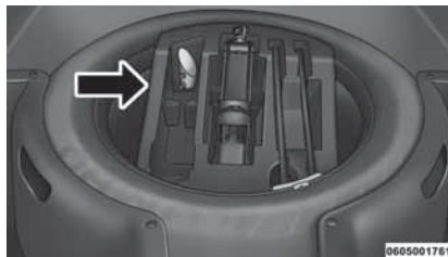
Jack Storage Location
