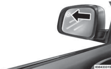
Warning Light Location
