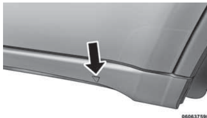
Lift Point Symbol On Sill Molding
