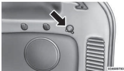
Rear Power Outlet
