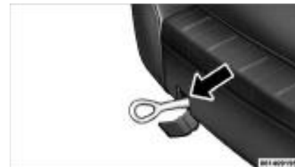
Rear Tow Eye Installed
