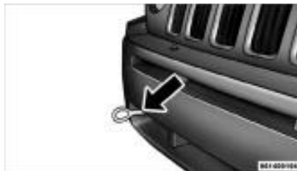
Front Tow Eye Installed
