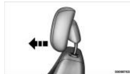
Active Head Restraint (Tilted)
