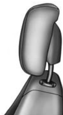
Active Head Restraint (Normal Position)
